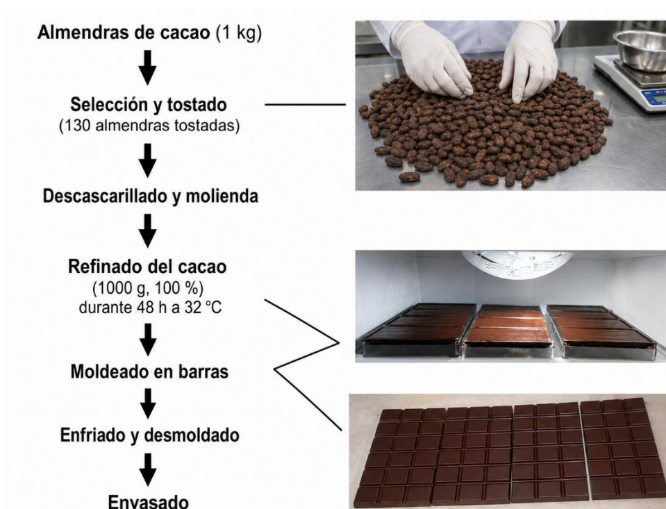
Figure 2. Diagram of the process for obtaining 100% cocoa paste.
